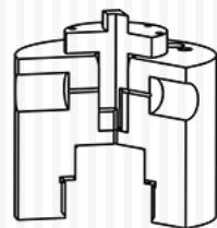
Valve design altered (two channels in the plug) to minimise the carryover volume inside the plug. Carryover volume of **1.4  $\mu$ L**.
