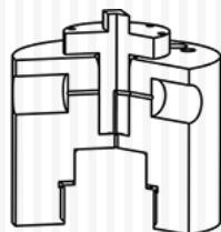
Syringe attachment modified to minimise the distance from the plug to the syringe. Carryover volume of **2.47  $\mu$ L**.
