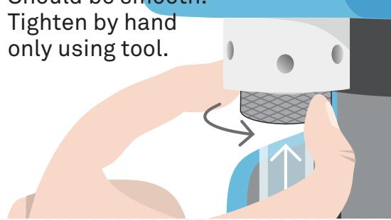
11 Move slider up using the driving wheel.
