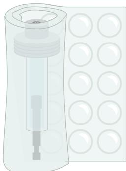
9 Check new syringe for cracks or fissures. Nothing should be seen. Check that o-ring is in place.
